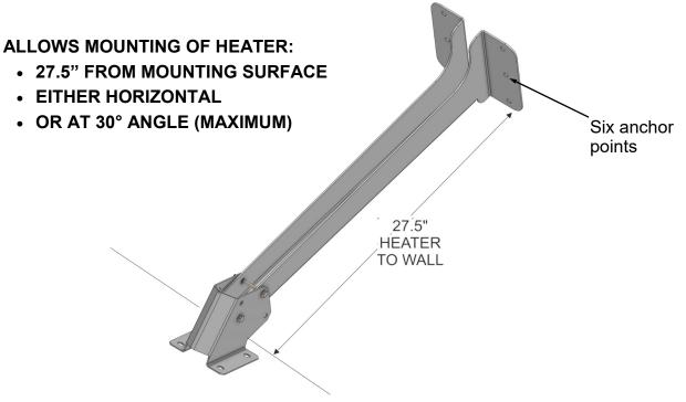
HEATER BRACKET FASTENS TO MOUNTING ARM WITH 2 EACH NUTS & BOLTS SUPPLIED
